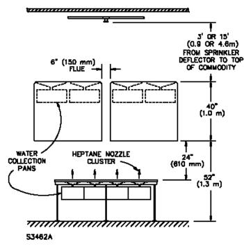
ADD testing is a useful tool to investigate a sprinkler's discharge characteristics; however, this testing is conducted with open sprinklers which does not investigate the potential for sprinkler skipping or blocked flues.
